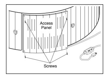
To replace the access panel, insert the top of the access panel under the edge of the spa shell. Slide the cover up until the bottom of the access panel clears the trim along the bottom of the spa. Then, slide the access panel into place and re-attach the four screws.
